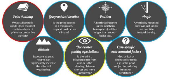
Outdoor durability of printed matter is defined by their resistance against different possible failure modes encountered in outdoor display. Typically, the following failure modes have been observed:
